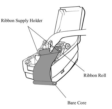
7. Put the print head module down and insert the bare core into the pick-up holder. (First snap in the left side, and then the right side.)
