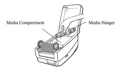
3. Load the media roll onto the hanger from left to right.
